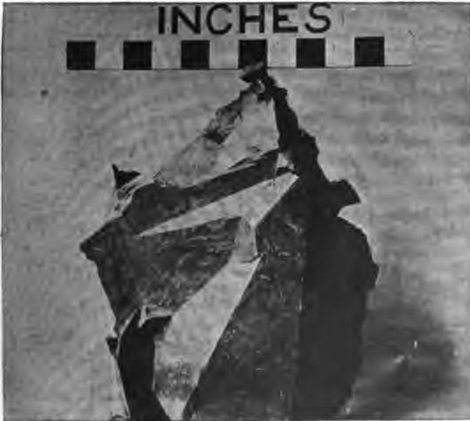
Fig. 39. Block of Ferromanganese with Large Facets Formed by Cementite Sheets. The Author's Collection.
